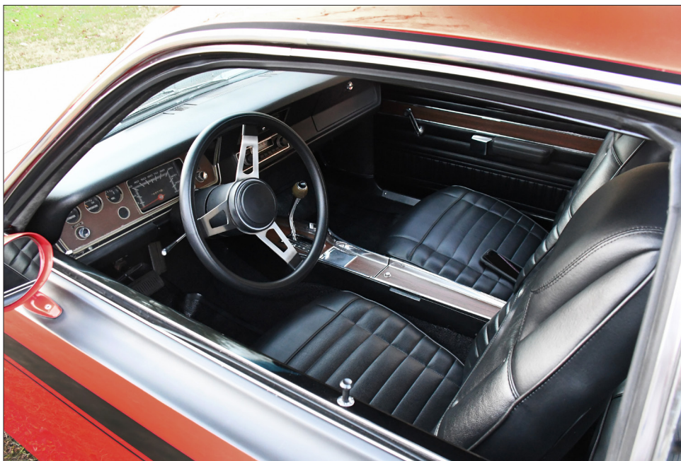
REHMERT HAD the dash and bucket seats, door panels and steering wheel replaced to match what a factory 340ci Duster would have been. The flat black hood sports a 340 wedge decal. The 340 "wedge" decal was introduced in '71. The wedge refers to the wedge cylinder heads which all 340s had.
